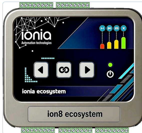
Front panel: four status LEDs and three buttons; the connection terminals are on the top and bottom edges of the housing.
